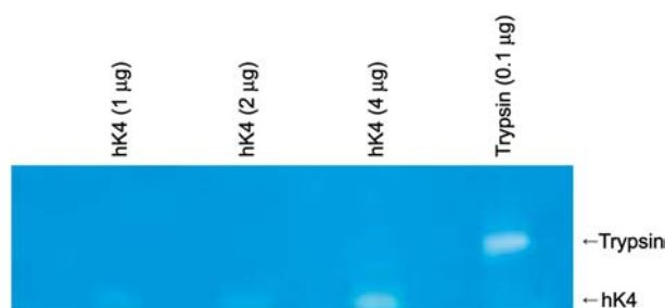
Figure 2 Zymography of 1, 2 and 4 \mu g of hK4 on a 10% gelatin gel stained with SimplyBlue™ SafeStain. Enzyme activity is indicated by clear bands. Trypsin (0.1 \mu g) was included for comparison.
