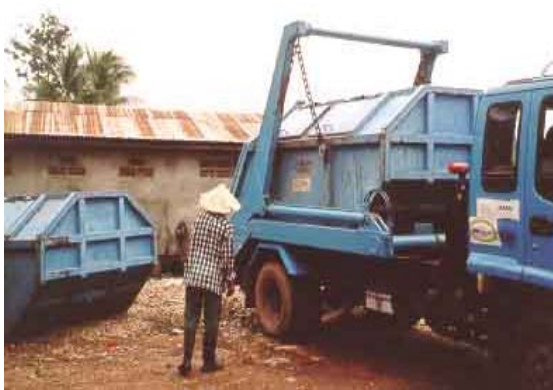
Figure 3.11: Hydraulic lift truck drops off empty bin and takes full bin to landfill
