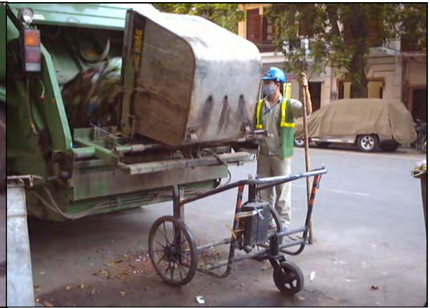
Figure 2.6 Hand-cart unloads organic waste into the truck after collecting this waste in small roads
